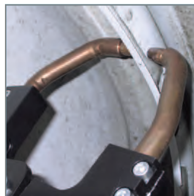
C-X adapter option can be used in applications where a C-type arm cannot reach.
